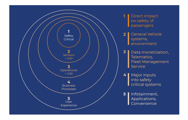
GuardKnox identifies 5 types of systems in the vehicle. Each type has identifiable characteristics and must be protected in accordance with its risk level.
