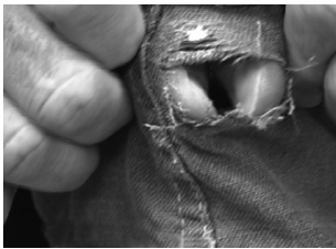
FIG. 2 Test fabric strength with thumbs
