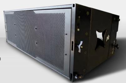
The high frequency section consists of three 1.75" planar wave drivers meticulously engineered to provide perfect acoustical coupling with adjacent cabinets, creating a continuous isophasic line source. Quad 6" neodymium, low distortion midrange drivers provide exceptional dynamic intelligibility.
