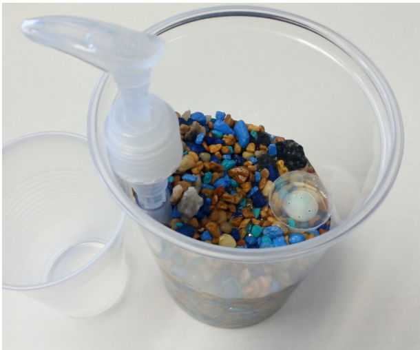
pumping water from the aquifer model
