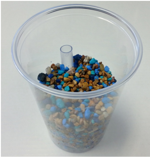
plastic container with large and small gravel layers
