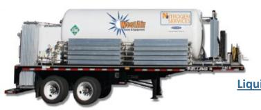
Gross Liquid Capacity 2,472 gallons Nitrogen Capacity SCF 218,620 Tank MAWP (psig) 600 Tank Overall Length 336 in. Tank Overall Height 78 in. Tank Diameter/Width 72 in.
