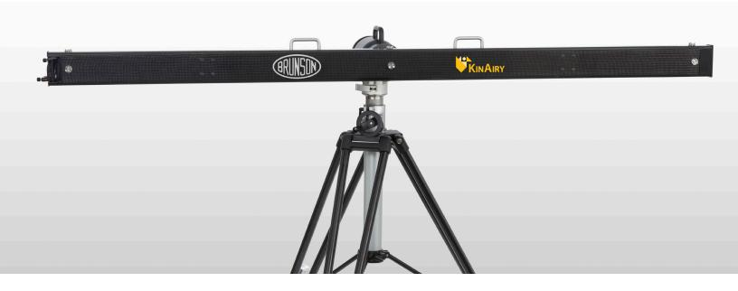
When seeking a NADCAP certification for Boeing, Models & Tools needed to demonstrate a periodic inspection procedure for their laser trackers. They turned to Brunson for a solution that included a NIST interim field test procedure and Maximum Permissible Error (MPE) report. Implementing Brunson's KinAiry system enabled Models & Tools to meet the challenge. They feel it improves their best practices and helps to minimize the frequency of non-conformances - and therefore future audits.
