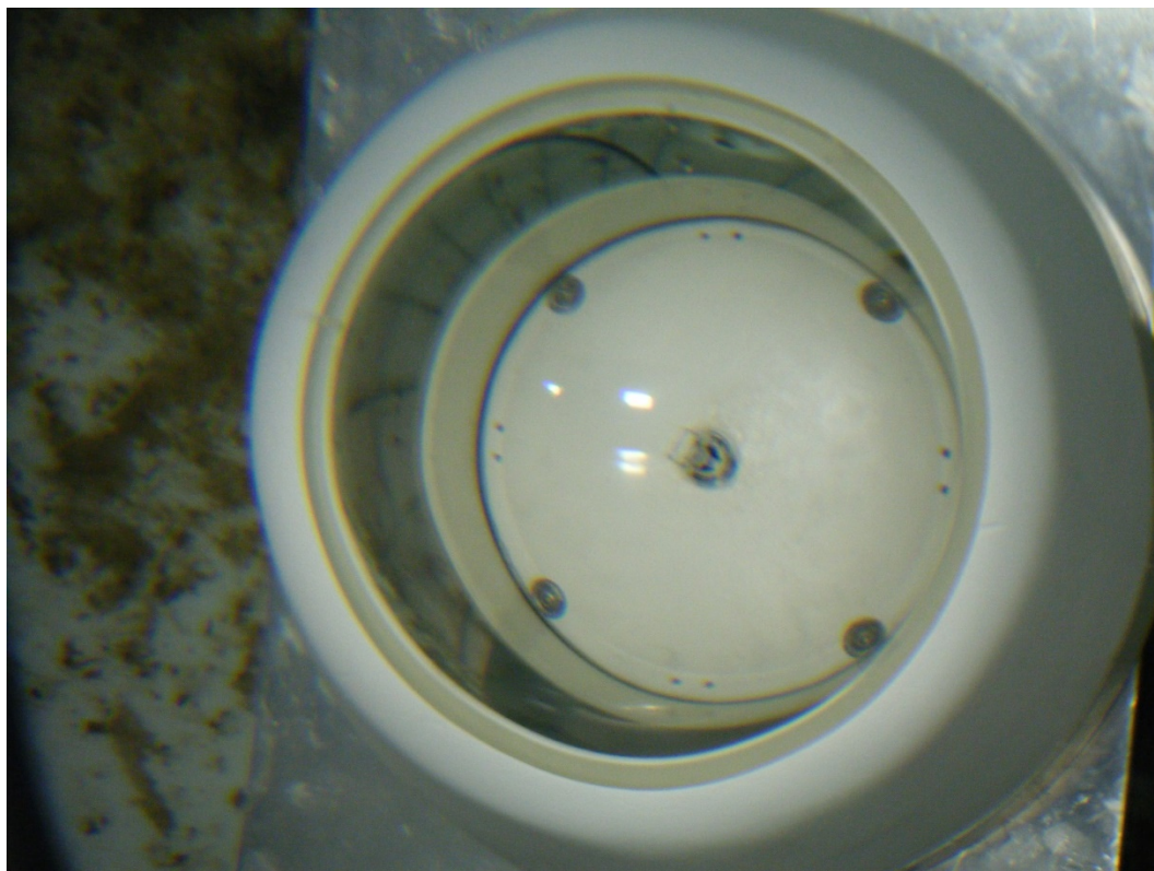
Test unit after water ingress test, no intrusion, completely dry on inside.
