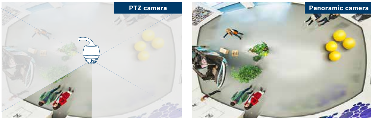
Fig. 6: Conventional PTZ camera view versus 360° surround view
