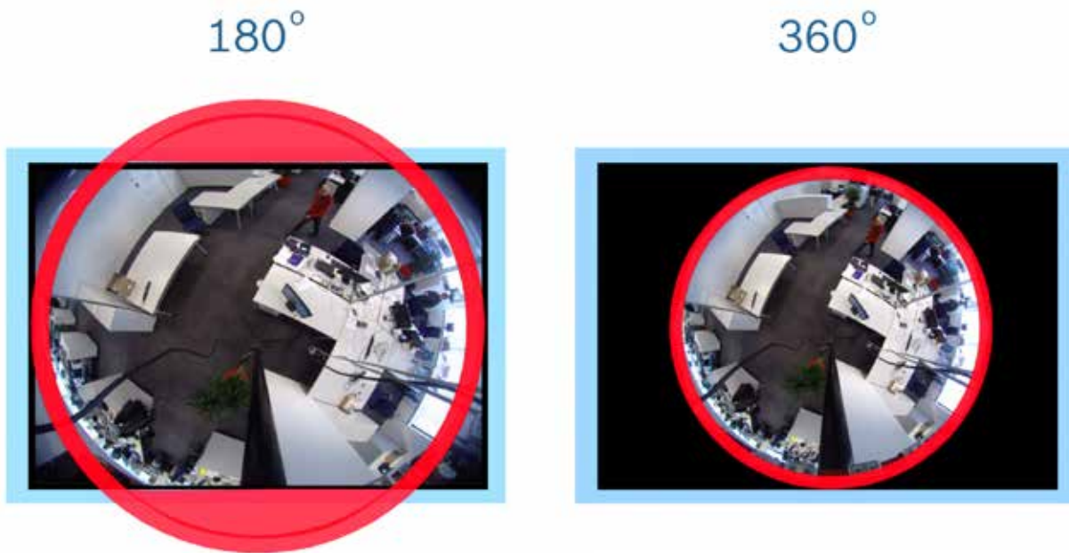
Fig. 2: Optical projection of a 180° and 360° lens
