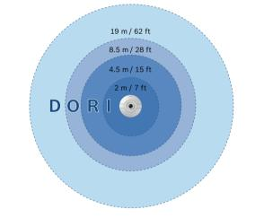
When mounted at a height of 3 m (10 ft) the 180° version of the camera has the following coverage radius for the four levels:
