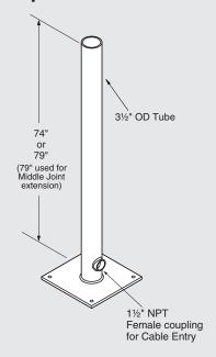
For use with a post top mount Vertica arm, the floorpost is a very popular method of mounting an arm when a structural surface is not available. The 74" post is for Vertica arms and the 79" post is for Vertica arms with a middle joint extension. Fabricated from heavy wall 31/2" structural tube welded to a 12" x 12" x 3/8" thick baseplate. A 11/2" female NPT coupling near the base for cable entry, additional couplings can be specified or located differently.
