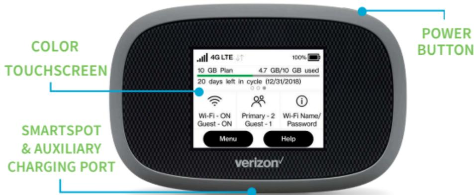
**POWER BUTTON:** Powers the Kajeet SmartSpot on and wakes the device from sleep mode.
