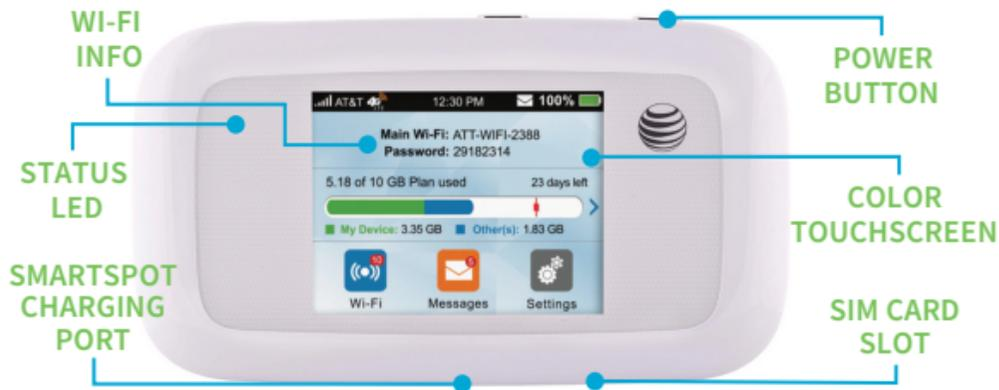
The Kajeet SmartSpot® is a portable Wi-Fi hotspot that extends the school day by providing the fastest, filtered broadband access outside the classroom.
