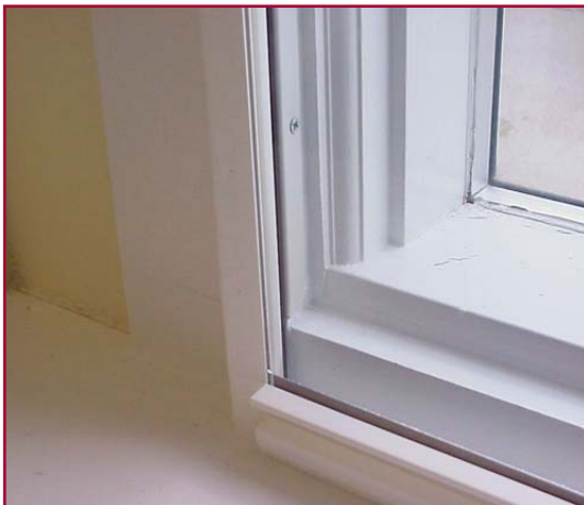
Shown above: FRAME ONLY – Surface mount style installation where the Climate Seal™ window is mounted on the surface of the existing window frame. This mounting style is preferred because of the increased amount of airspace, which allows for maximum sound reduction between the existing
