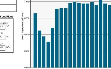
Sound Absorption Coefficient vs. Frequency
