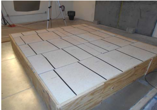
E400 test with 5/8" Envirocoustic Wood Wool (2" backing)
