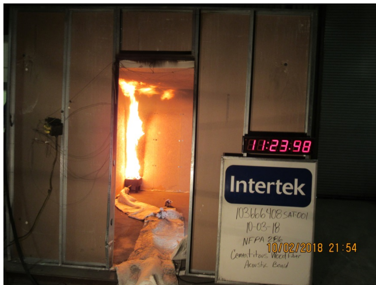
Photo No. 8 160kW
