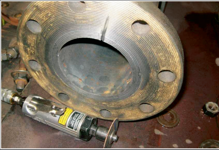
APT used a pneumatic grinder with an abrasive wheel to simulate severe "impact damage" 0.100 inches in depth.
