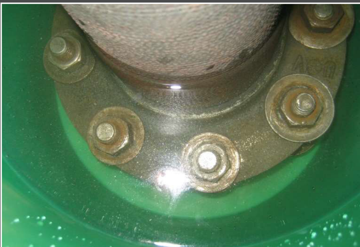
The spool piece was pressurized to 100 psi for 8 hours and the connection stayed "bubble tight".
