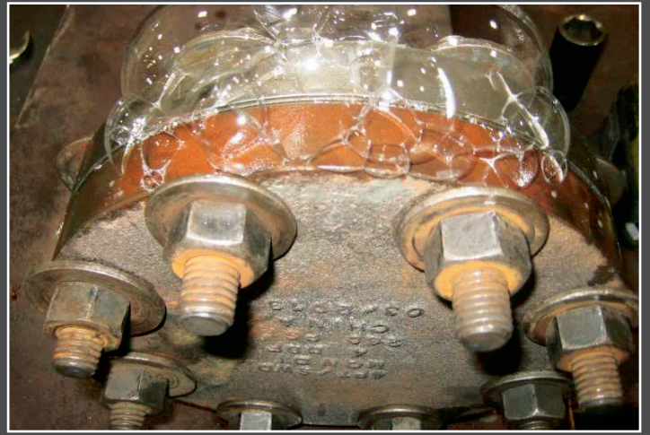
As the soap solution shows, the gasket was unable to seal the "damage" and prevent a leak.
