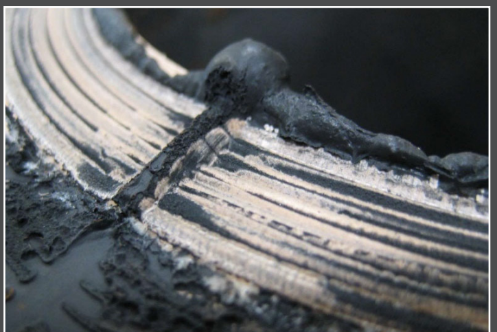
The Flange Pelseal ® filled the depth of the damage, which exceeded the deformation limits of the Step-Ring gasket, bonding well with both the MONDI™ and the gasket.
