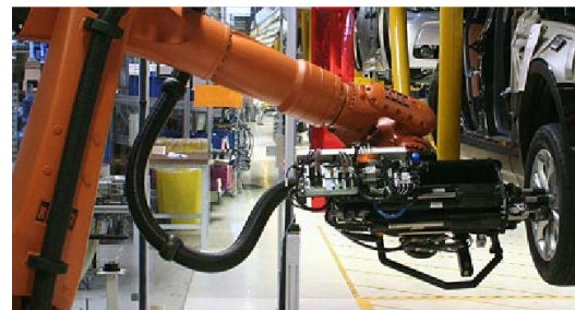
Figure 1: The assembly system mounts wheels onto the continuously moving vehicles
