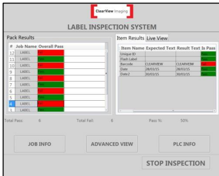
Figure 1: Screenshot of the inspection system working in real time
