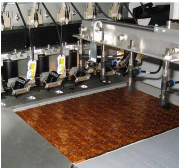
A flexible printed circuit panel is shown on the vacuum platen, in front of the five inspection cameras and LED light sources.
