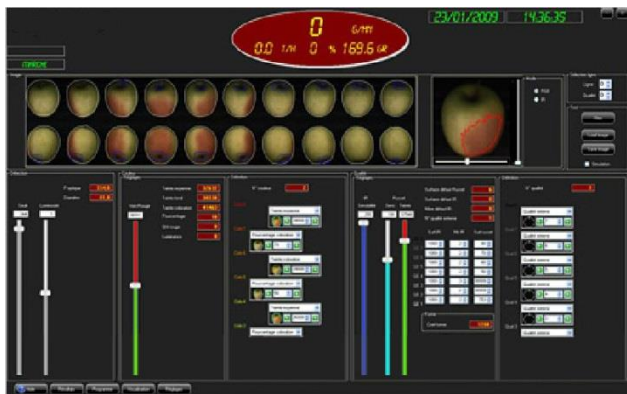
A 3D display provides the operator with information on a piece of fruit's size, colour and any defects.
