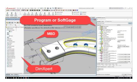
CheckMate programs used to drive coordinate measuring machines and as soft gauges for use with point cloud data from laser scanners are generated using MBD pulled from the DimXpert tree
