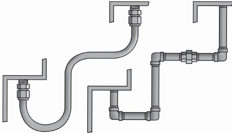
Whether it's a new construction or a retrofit, power plant tolerances can be tight. Swagelok offers small bore (up to 2 in. [50 mm] O.D.) tubing solutions to lessen the amount of installation space needed. Using tubing also improves safety by eliminating the need for welding in hazardous environments. And small bore tubing reduces the number of connections and potential leak points to improve fluid flow through the system. [Learn more about Small Bore.](#)
