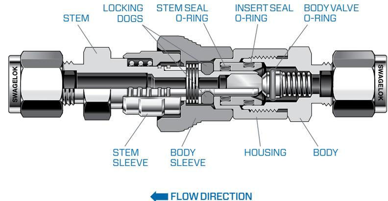
Simplify your installation even more—and still ensure fluid system integrity with Swagelok Quick-Connects. Push-to-lock connection means no tools or wrenching necessary. [Learn more about our Quick-Connects.](#)
