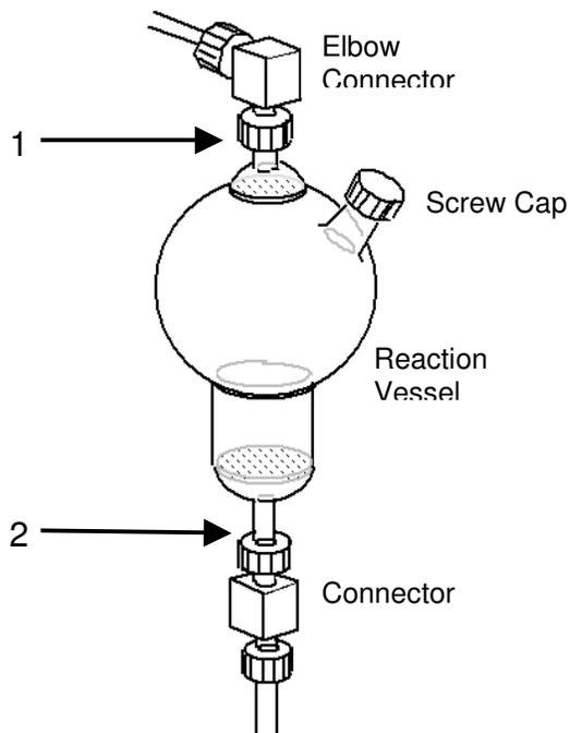
1. Place RV top flush into top connector. Tighten connector hand tight.
