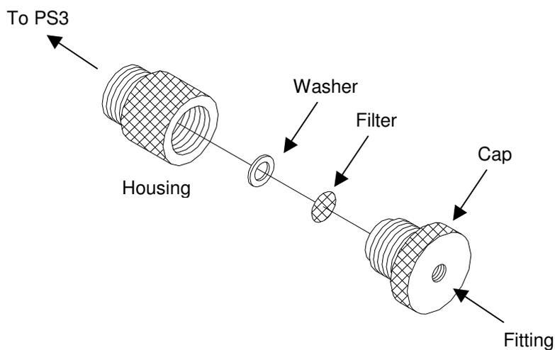
2. If the filter is dirty, remove the washer and filter from the cap and wash with ethanol to remove particulate matter.
