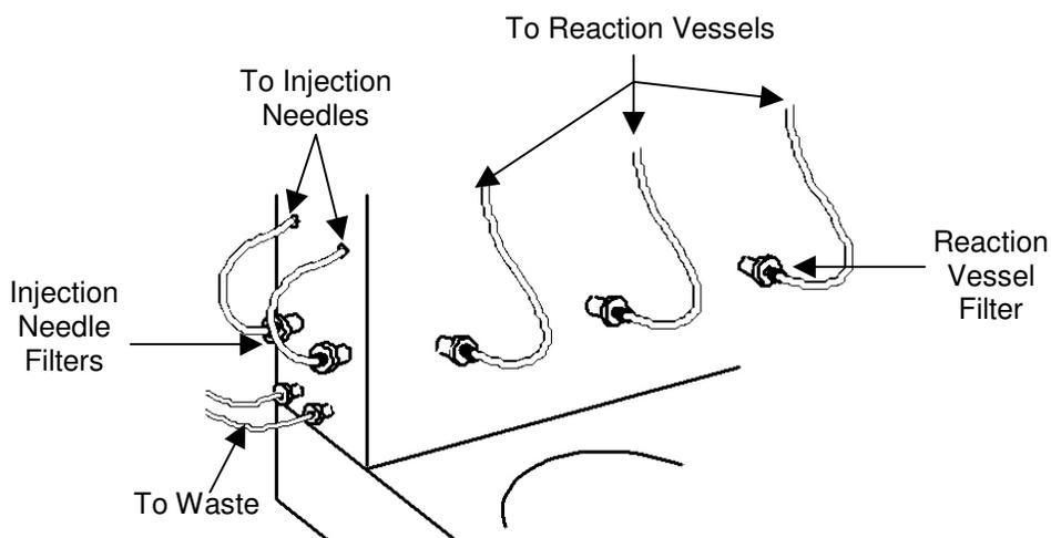
To check inline filters for particulates:
