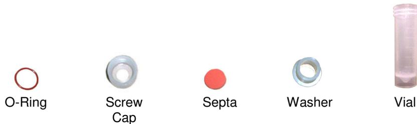
To assemble the capped vial:
