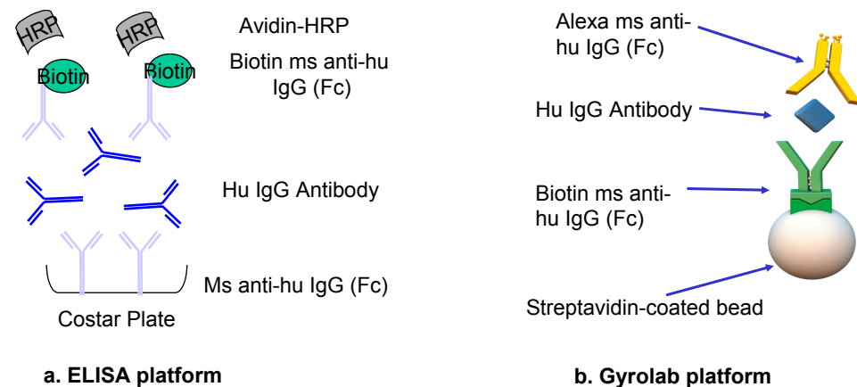
Figure 2: Schematic of the Generic Assay for the Quantitation of Human IgG in Rodent Serum in: a) an ELISA platform, b) the Gyrolab platform
