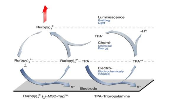
MSD® is a plate reader based on electrochemiluminescence (ECL) detection technology using Sulfo-Tag labels. Multiple analytes can be measured in the same well.
