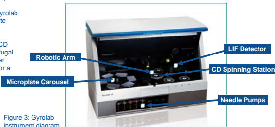
Figure 3: Gyrolab instrument diagram
