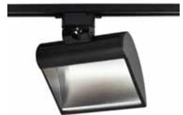
**MAC LED TRACK** Nora MAC LED Track Series offers two luminaires: MAC, 700lm (10W) and MAC XL, 1100lm (18W). Fixture has a sleek, driverless appearance and field changeable beam spreads. Pre-installed narrow flood optic is included, along with an additional spot optic. 2700K to 4000K at 90+ CRI.
