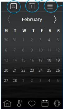
A magnetic contact must be connected to the door (Tylö part no. 90908035) in order to use the calendar functions for the Sauna and Combi heaters, and also the Tylarium system.
