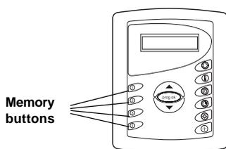
When the control panel is delivered from the factory the memory buttons are pre-set. It is a good idea, however, to change the settings so that you get the sauna bath of your choice. Set the temperature and duration of the sauna heater according to earlier instructions (see page 10).
