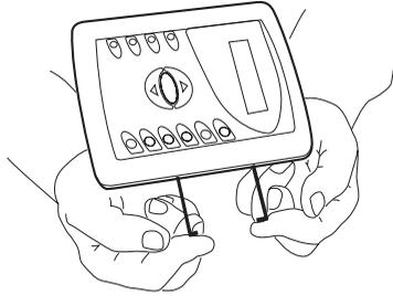
*Open the lid of the control panel by inserting the control panel openers on the side.*
