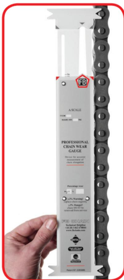
Place one 'V' jaw of the instrument over the first pin of the selected sections and then extend the slide until the other 'V' jaw reaches the nth (as previously determined).
