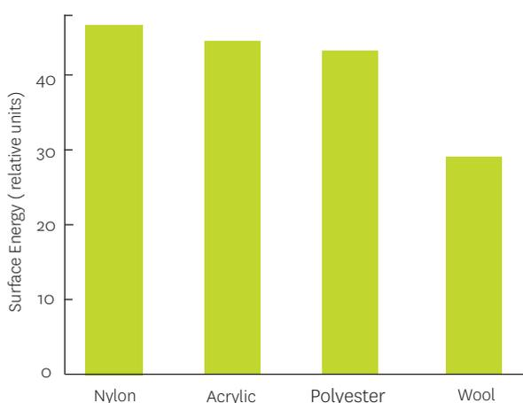
Figure 1. Fibre surface energies for various fibres (Leeder, 1984)
