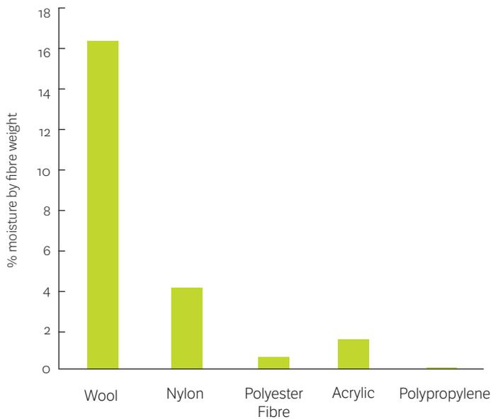
Figure 2. Moisture absorbance of wool and synthetic fibres (Collie and Johnson, 1998)
