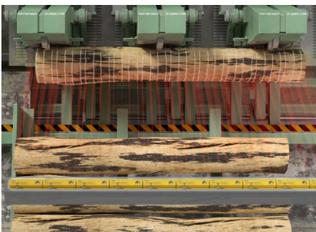
A bank of chroma+scan 2400 series multi-point scanners snapshot scanning logs in a carriage system.
