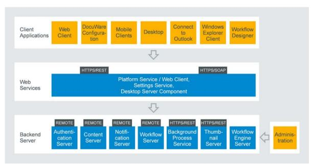
Communication between the layers of client applications, Web Server, and backend server
