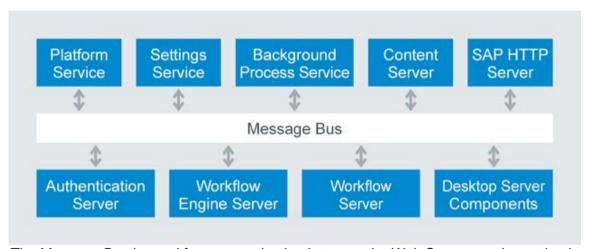
The Message Bus is used for communication between the Web Servers and most backend servers.
