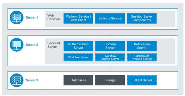
DocuWare system with separate machines for the backend servers and for databases, fulltext functionality, and storage locations
