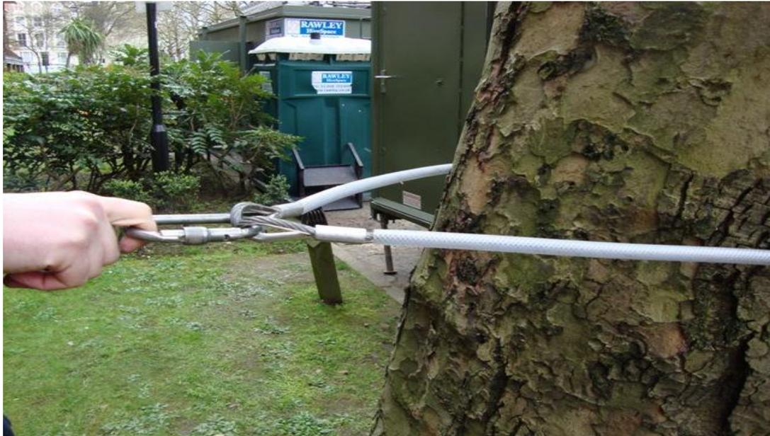
Photo 1: Strop set up as a Primary Anchor. There were four of these together to anchor four ropes.
