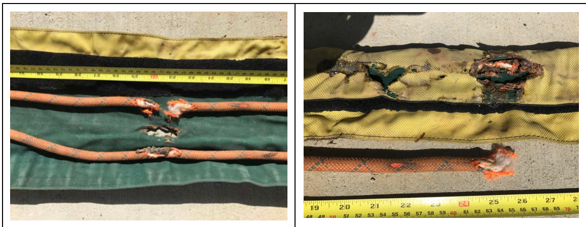
Figure 2: Damaged ropes and rope protector
