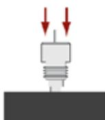
flat surface to reshape the seal. Flip seal over and repeat. If the swivel continues to leak, return for factory service or order replacement seals.
