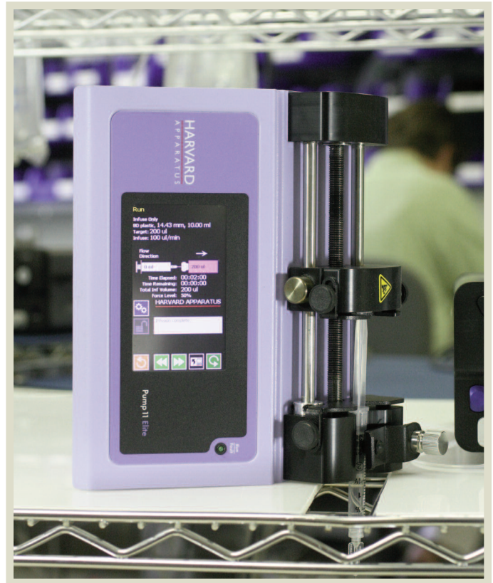
The touchscreen on all 11 Elites can be rotated so that you can orient the pump vertically to save benchtop space and allow gravity to clear air bubbles. (Shown here on a rack configured for infusion and automated blood sampling.)
