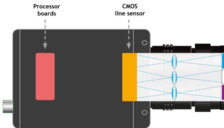
*This method uses line scan sensors where the horizontal resolution of the sensor can be divided into multispectral domains by adding additional filters in the optical assembly. Here a trilinear sensor is divided into three spectral separations resulting in a 9-channel multispectral camera.*
