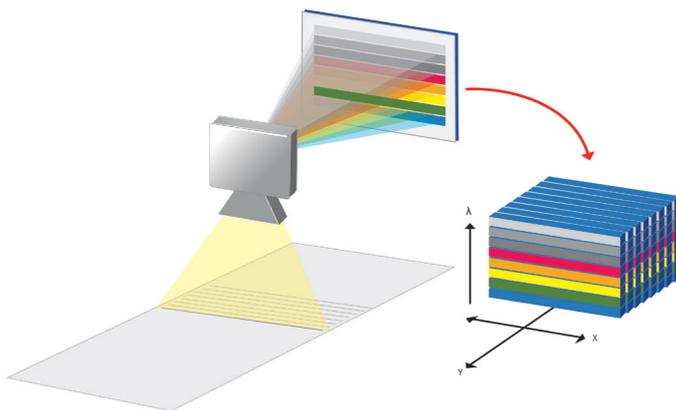
*It is possible to do multispectral imaging with the Pushbroom hyperspectral camera technique, where full spatial and spectral information is captured line by line.*
