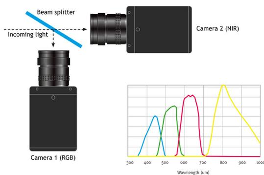
This multispectral imaging technique uses a beam splitter. Hence, it is possible to simultaneously capture images using multiple cameras.
