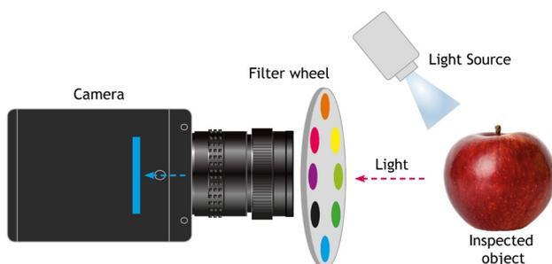
*A multispectral camera using filter wheel captures multi-spectral images. This is done by rotating the filter wheel mounted in front of the lens or in-between the sensor and the lens.*
