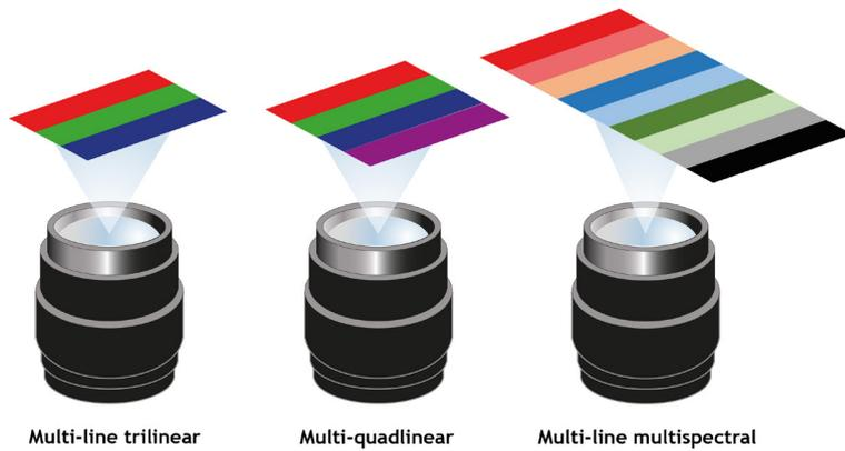
*Line scan cameras with multi-line sensors can be used for multispectral applications, where each line of pixels has a unique spectral band-pass filter.*
