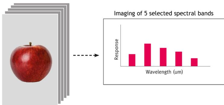
*Multispectral imaging consists of spectral bands which are discretely positioned from each other. In other words they do not provide a continuous spectrum.*
