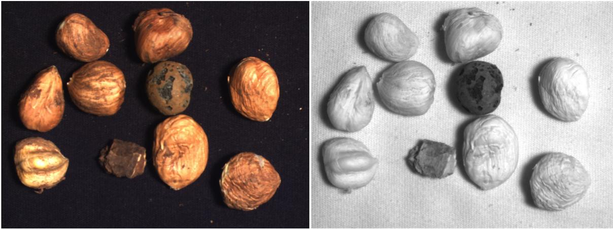
*In this example, foreign objects are located during the inspection of hazelnuts. These foreign objects absorb higher energy in NIR and therefore appear darker in the NIR image. The difference between foreign objects and hazelnuts is less visible in the RGB color image.*
