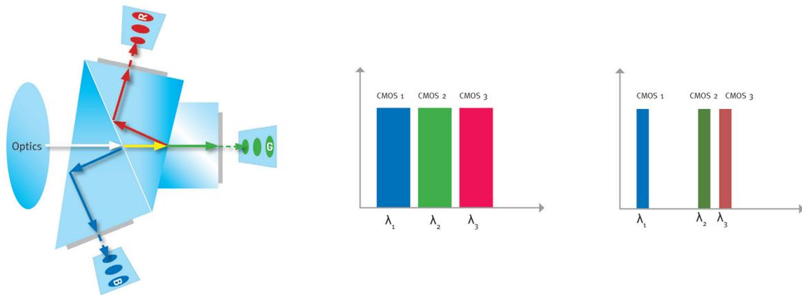
*In prism-based cameras, the prism blocks consist of hard dichroic coatings which are interference filters by nature. These filters are responsible for the primary separation of incoming light.*
