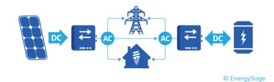
Example of AC-coupled system: DC electricity flows from solar panels to an inverter that transforms the energy to appliancefriendly AC. To store it in a battery for later use, it will need to flow through another inverter, transforming it back into DC.
