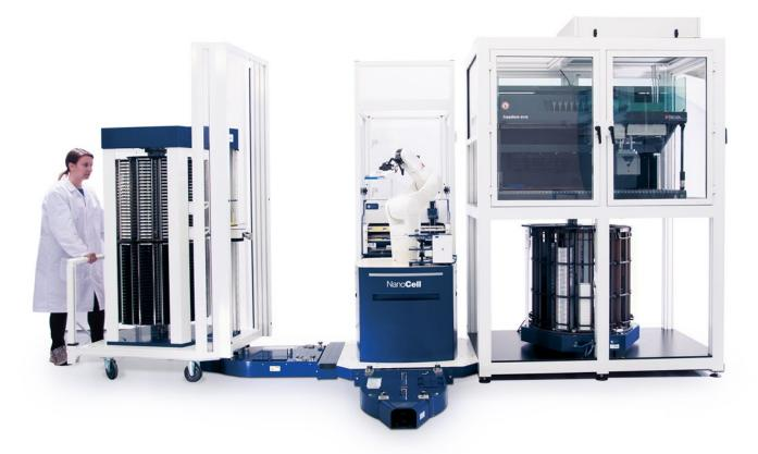
These systems along with their associated devices are controlled using the HighRes Cellario dynamic scheduling application. Mosaic interfaces with Cellario using Titian's Cellario Fulfilment Module (CFM) to allow order creation and workflow tracking.
