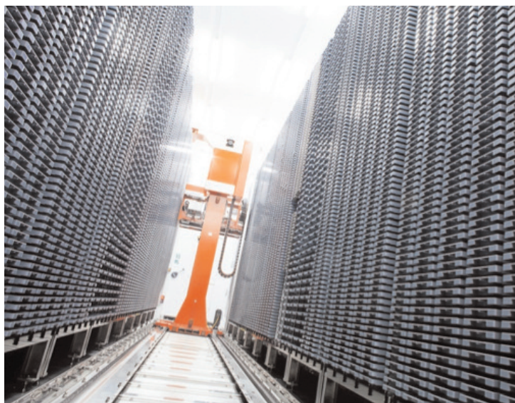
REMP LSS (Large-Size Store) with 80 Million \mu Tube capacity and -20°C \mu Tube picking robot
