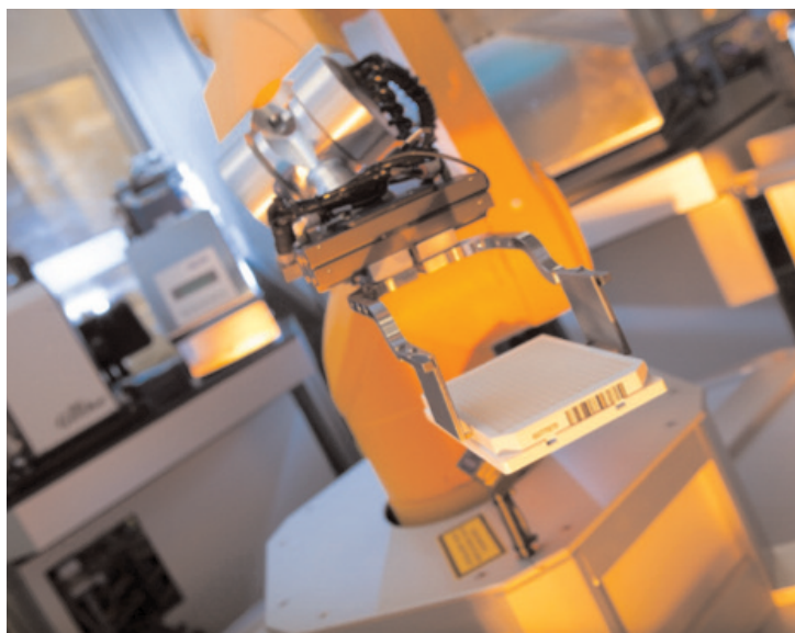
Stäubli Robot arm moving a REMP \mu Tube plate in a dehumidified environment
