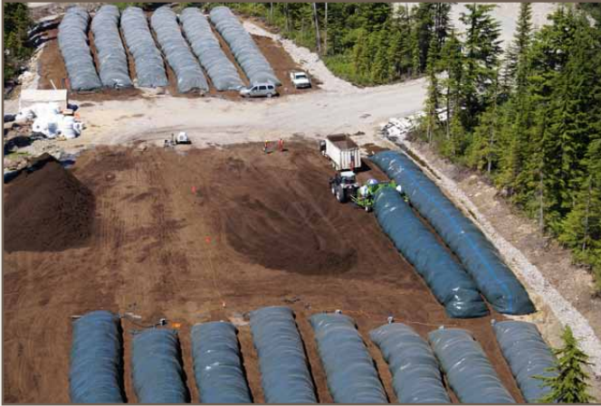
Raw compost is completely enclosed in AG-BAG eliminating leachate and odor issues. Compost under positive aeration. Temperature is monitored under OMRR regulation.
