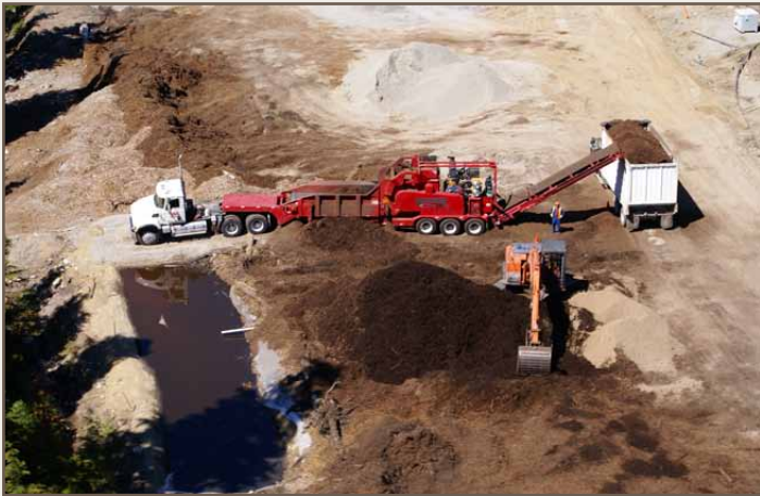
On-site grinding of land-clearings that would have been burned or buried. Mixing-grinding of wood waste (carbon) and nitrogen source prior to composting
