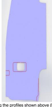
Cut along the profiles shown above (located on the back of the panel) to use in 2018 or earlier model years
