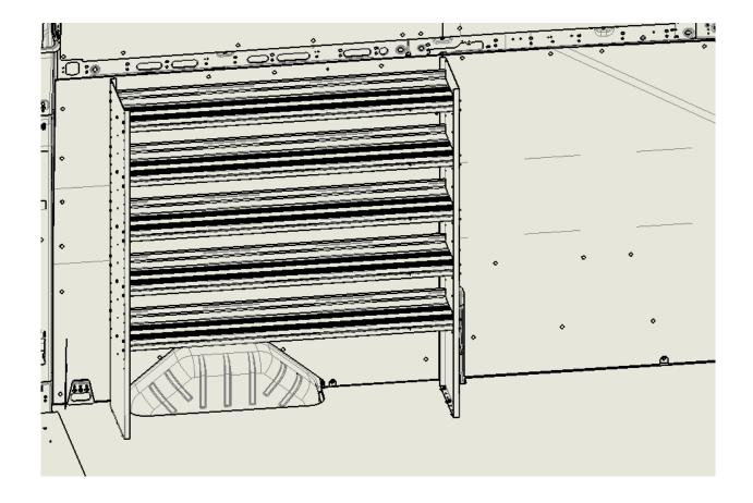
The plastic floors expand and contract depending on what the temperature is in the environment, the floors must Not be clamped down and prevent this expansion and contraction from happening, the floor must float at all times, if not, it may become wavy and bumpy which will be very uncomfortable and a trip hazard for your customer.
