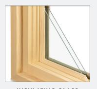
INSULATING GLASS Our standard glazing is Insulating Glass (IG) with Low E2 and argon gas. IG glass is double glazed and compared to a single glass pane, cuts heat loss significantly because of the insulating air space between the glass layers.
