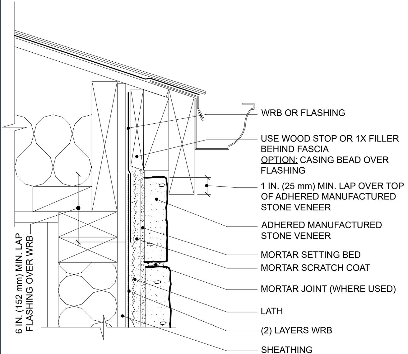
Water resistive barrier should be in place prior to soffit installation followed by adhered manufactured stone veneer.
