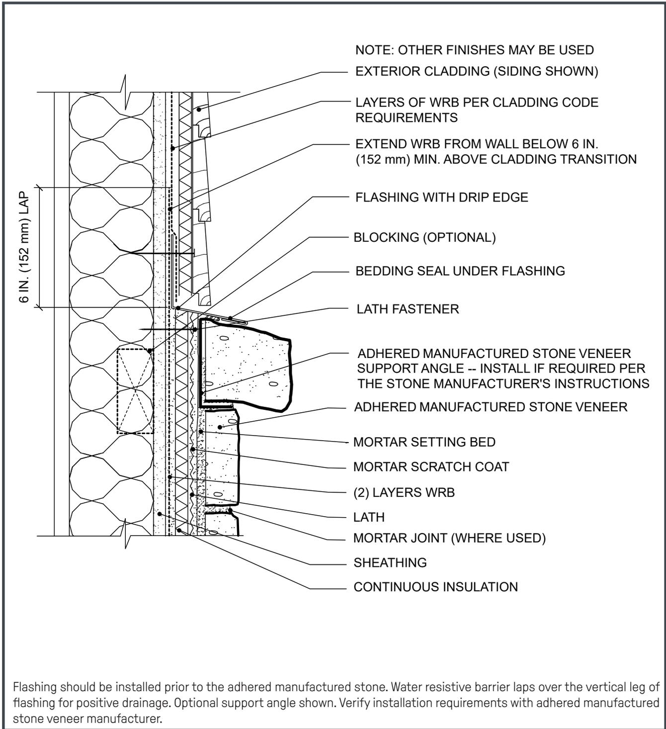
Flashing should be installed prior to the adhered manufactured stone. Water resistive barrier laps over the vertical leg of flashing for positive drainage. Optional support angle shown. Verify installation requirements with adhered manufactured stone veneer manufacturer.
