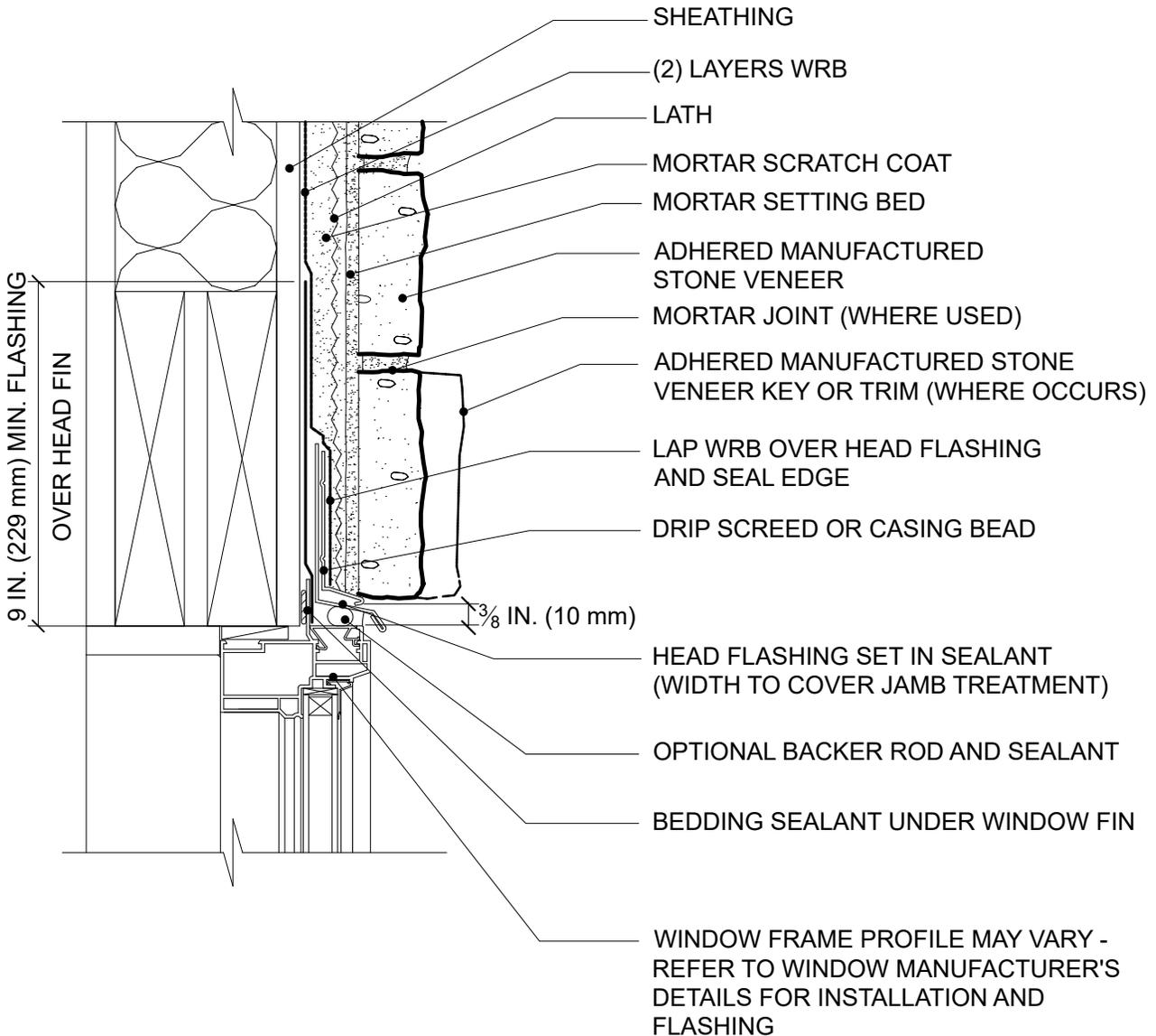
Flashing and WRB installed shingle fashion may be complimented with self-adhered flashing (SAF) to seal WRB to window frame.
