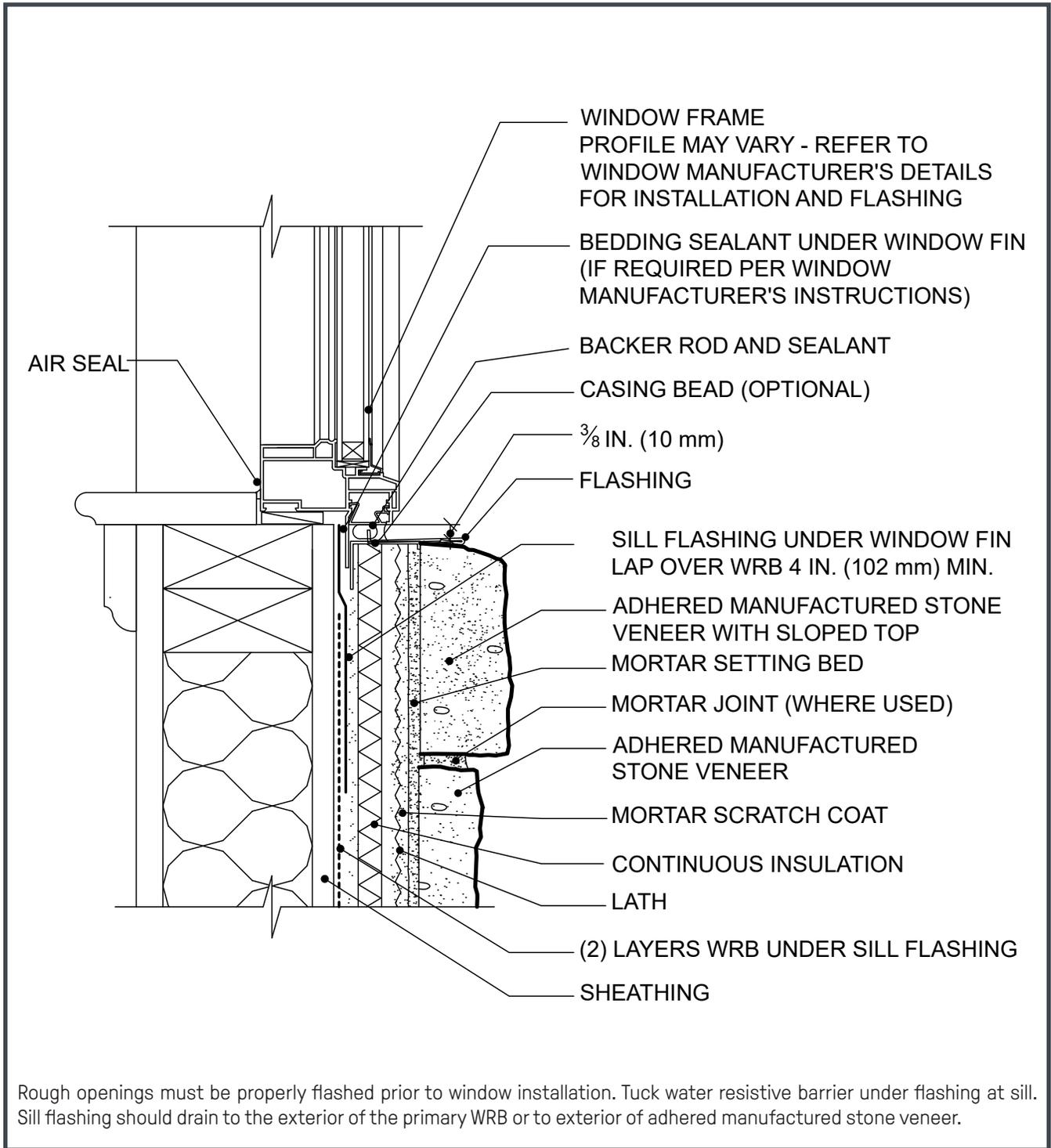
Rough openings must be properly flashed prior to window installation. Tuck water resistive barrier under flashing at sill. Sill flashing should drain to the exterior of the primary WRB or to exterior of adhered manufactured stone veneer.
