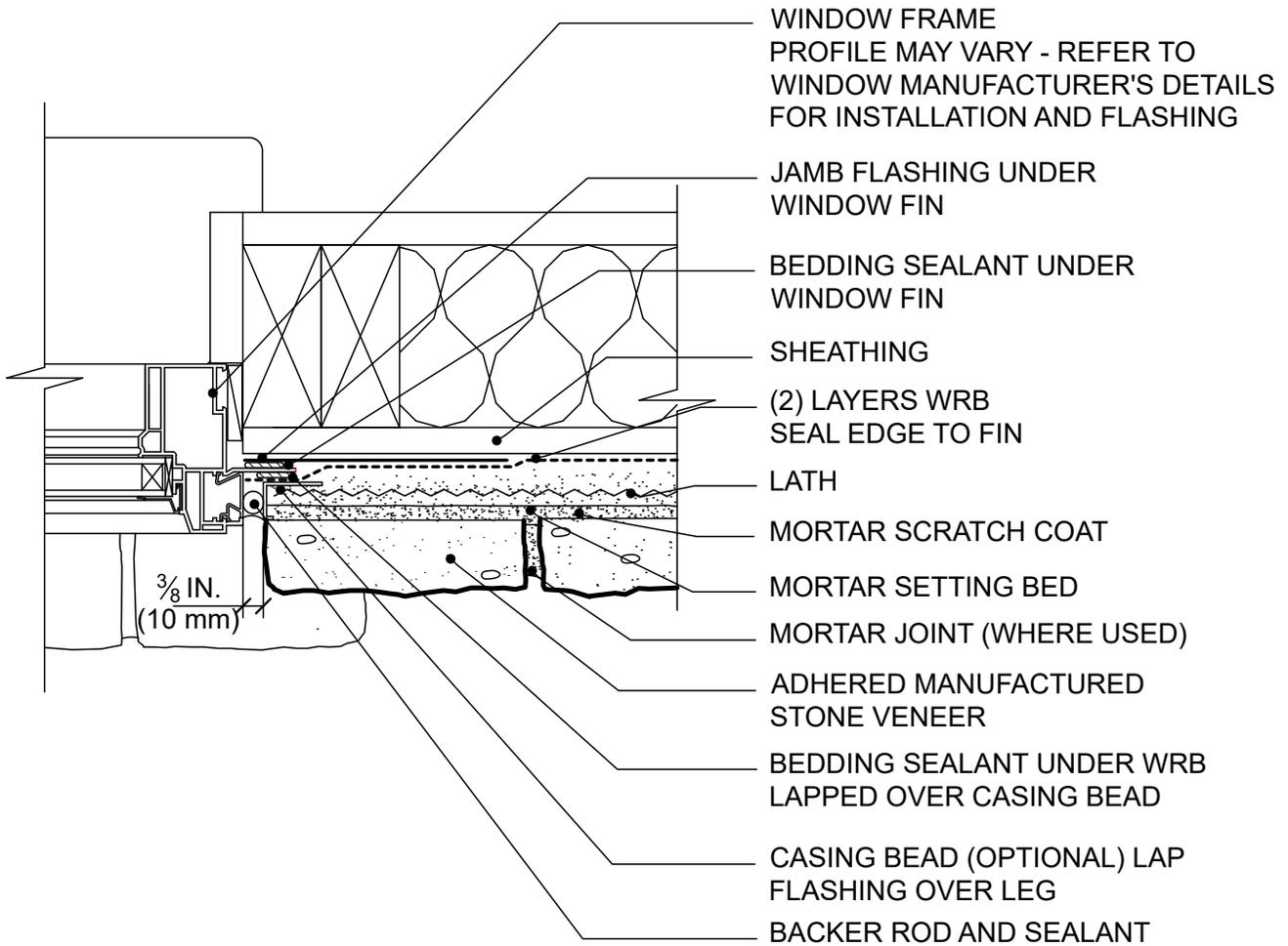
Rough openings must be properly flashed prior to window installation. Backer rod and sealant between the window frame and the adhered manufactured stone veneer allows for movement between the dissimilar materials.
