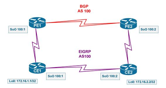
In this case, SoO communities are applied on the PE-CE links as well as on the backdoor link. When a route flaps inside the VPN site, stale information is stopped from ever looping back to the origin as following:
