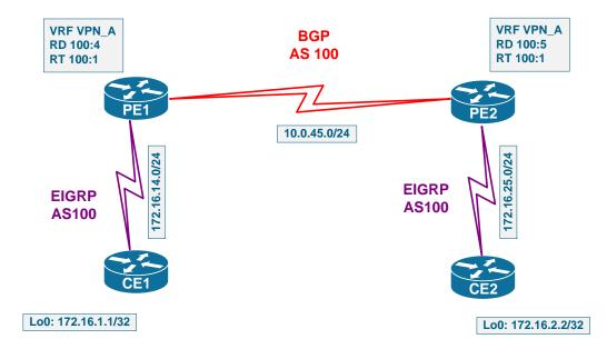
Here PE1 and PE2 redistribute between EIGRP AS 100 process for VRF VPN A and BGP process for AS 100. The redistribution process is slightly different than it would have been if no VRFs were present. In short, this is what happens when CE2 advertises the prefix 172.16.2.2/32 into EIGRP
