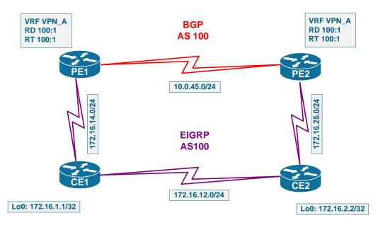
There could be certain race conditions in the above scenario, based on the timing of EIGRP/BGP updates. Race conditions are not uncommon in gradient algorithms, which accept best information instantly, based solely on the local decision. This behavior is non-deterministic may lead to some unwanted or even dangerous behavior.
