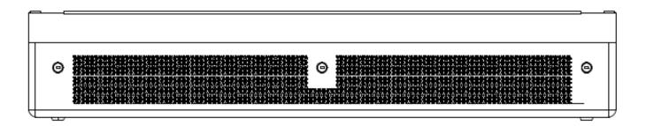
**Please note:** The grille size used in an IP3x anti-ligature radiator guard can inhibit the convection process. Therefore Contour cannot guarantee that the casing will not exceed a surface temperature of 43 degrees Centigrade.
