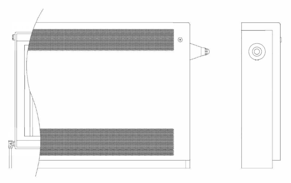
**Please note:**The grille size used in the IP3x anti-ligature radiator guard can inhibit the convection process. Therefore Contour cannot guarantee that the casing will not exceed a surface temperature of 43 degrees Centigrade.
